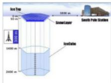
Diagram of IceCube. IceCube will occupy a volume of one cubic kilometer. Here we depict one of the 80 strings of optical modules (number and size not to scale). IceTop located at the surface, comprises an array of sensors to detect air showers. It will be used to calibrate IceCube and to conduct research on high-energy cosmic rays. Author: Steve Yunck, Credit: NSF
