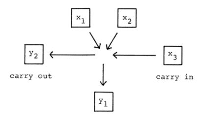
If each bit  $x_1$ ,  $x_2$ ,  $x_3$ ,  $y_1$ ,  $y_2$  is interpreted as a variable over  $\mathbb{Z}/2\mathbb{Z}$ , then the above adder is represented by the equations
